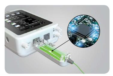
Each sensor module stores calibration data in its own local memory, that LEO reads upon connection.
